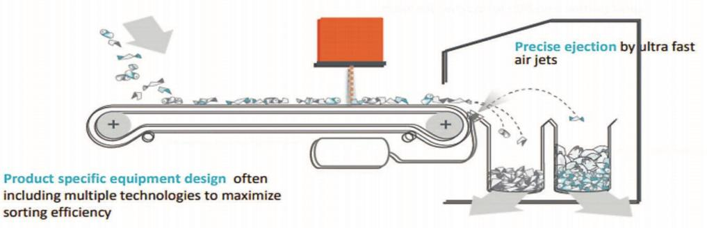
High-speed processing of information (material, shape, size, color, defect, damage and location of objects)
